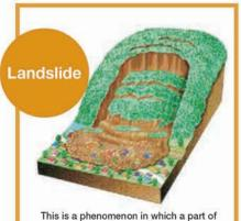
a mountain or slope gently moves downward while retaining its original shape to some extent. This is caused by rising groundwater levels due to rainfall and melting snow, or by human-induced topographical changes.
